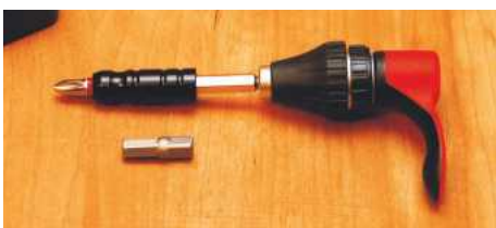
▲ Alternatively it will take the magnetic bit holder to extend it
